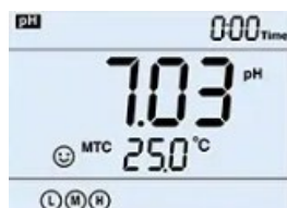
The large backlit LCD display pH and temperature simultaneously along with icons of stable readings and finished calibrations.
